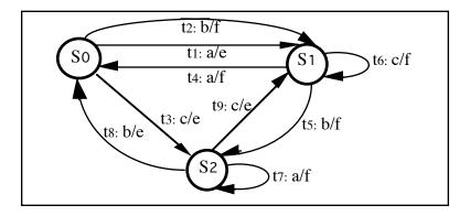
Figure 1: A state transition diagram of an FSM
