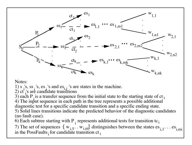
Figure 6 : Construction of additional diagnostic tests
