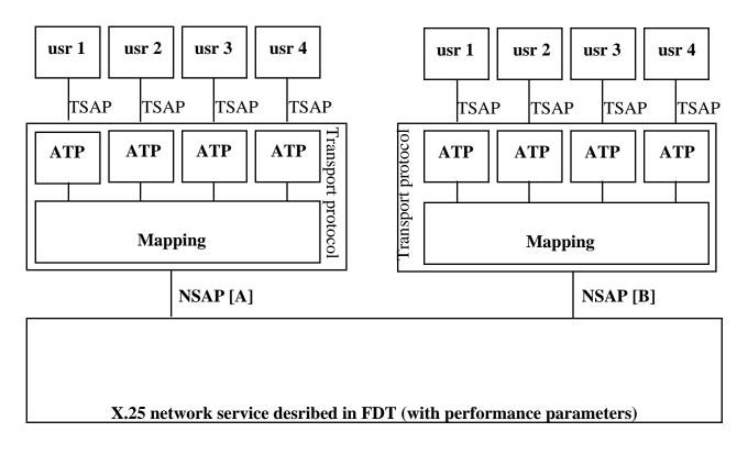
Figure 5- FDT simulation module with Transport protocol
