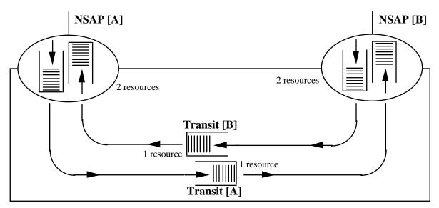
Figure 4- Structure of the Network module specified in the Annex
