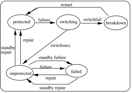
Figure 5: Initial system specification.
