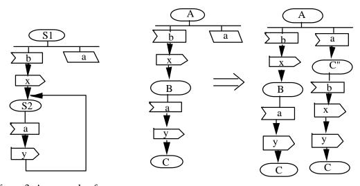
Figure 3. An example of an SDL-mchine without equivalent FSM
