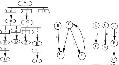
Figure 11. An example of an SDL-machine
