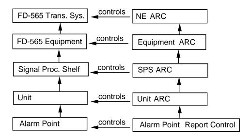
Figure 4: Alarm Report Control (ARC) support objects
