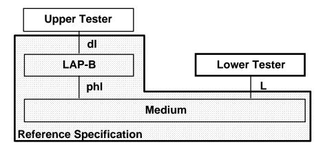
**Figure 3. Remote Test Architecture**
