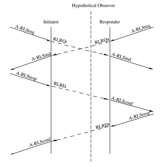
Figure 4. Sequence of ASPs and APDUs in the release collision scenario
