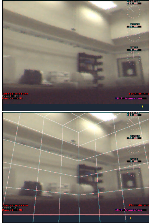
Figure 5: Immersive viewing with an HMD (top left) of a section of a panorama generated from a panoramic camera image (top right). The user sees a pinhole projection model image (bottom) in the HMD screen created from the image cube form of the panorama data.
