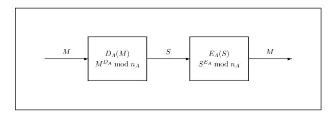
Figure 5: Message authentication using RSA algorithm
