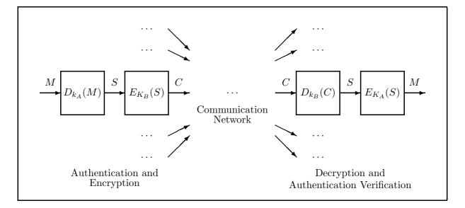
Figure 3: Communication link with public key authentication and encryption
