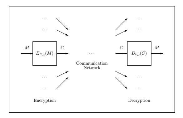
Figure 1: Communication link with public key encryption
