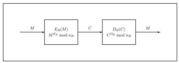
Figure 4: Block diagram of RSA secure communication link
