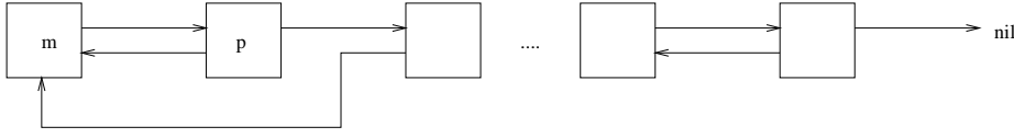
Fig. 3. When processor p gets a positive response from its successor to p 's delright query, p 's successor updates its own predecessor in the shared list. In this case m is that predecessor. Thereafter m should update its own variable to point to the head of the shared list.
