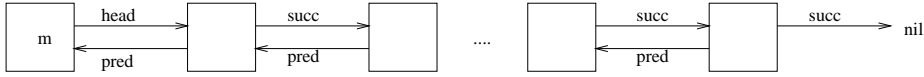
Fig. 1. In an idealized view, memory and processors which have indicated to read or write the cache form a doubly linked list.
