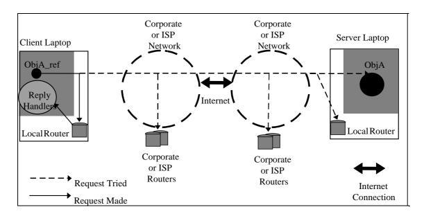
Figure 22-2 TII: No direct connection possible
