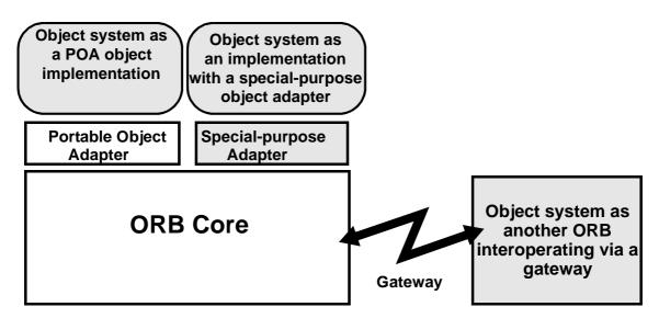
Figure 2-9 Different Ways to Integrate Foreign Object Systems
