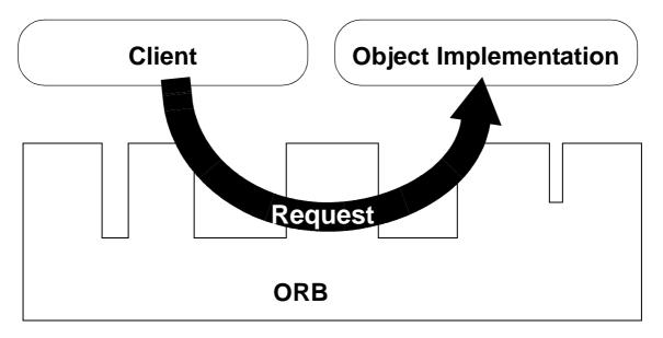
Figure 2-1 A Request Being Sent Through the Object Request Broker
