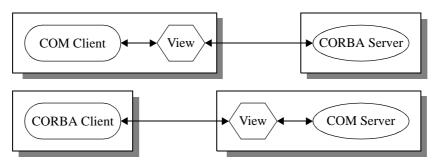
Figure 20-1 COM/CORBA Part A Configurations
