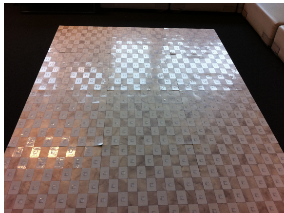
Fig. 6. Layout of RFID tags on the floor
