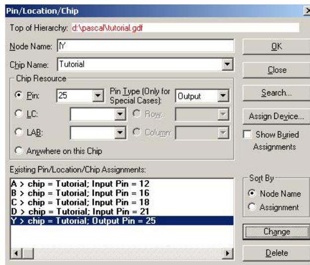
Figure 5 Pin/Location/Chip window
