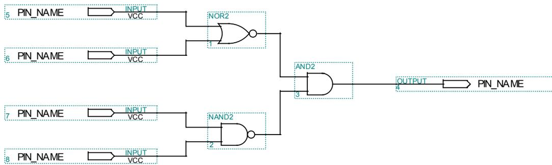
Figure 3 Schematic with input and output wired
