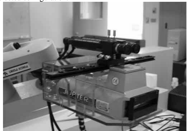
Fig. 1: Multi-modal chassis attached to the robot end effector.
