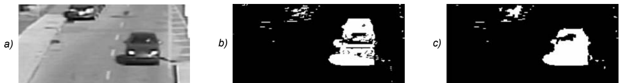
Fig. 5. Effect of ghost pixels on binary mask: a) initialization image, b) mask with ghost pixels, c) mask after ghost removal.
