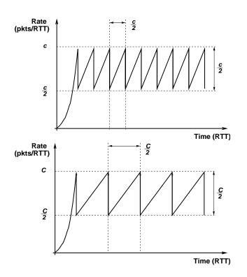
Table 1: Characteristics of a 200ms TCP connection using traditional congestion control.
